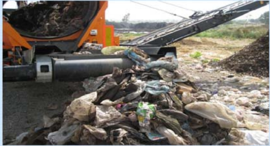
Fauji Cement: pre-screening
