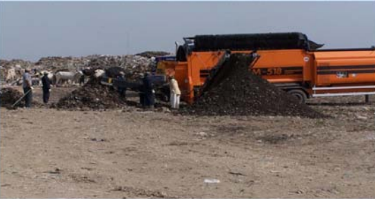
Fauji Cement: separation of inert / sand
