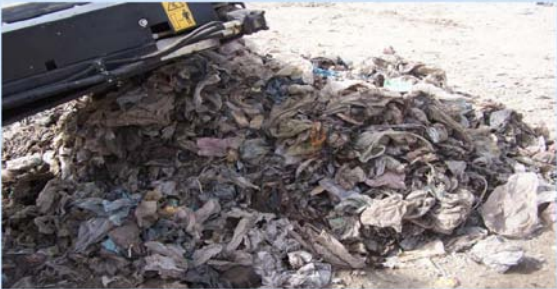
Fauji Cement: oversized consisting of plastics
