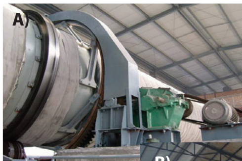
Figure 1: A and B) A 100kt/y gypsum line producing phosphogypsum for Jinshan Dawei Co, Sichuan Province; C) Kiln used by ESEC
