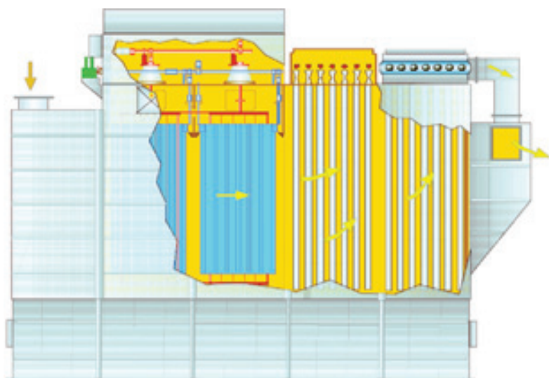
Below: The ESP and fabric filter (FF) section of the hybrid filter.
