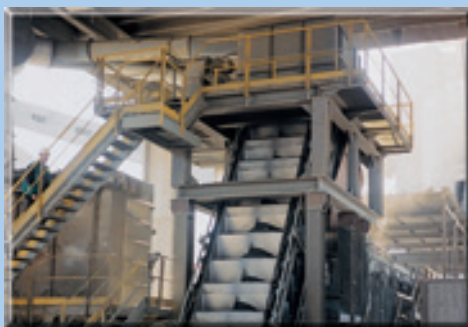
Deep bucket clinker conveyor for material handling with considerable inclinations.
